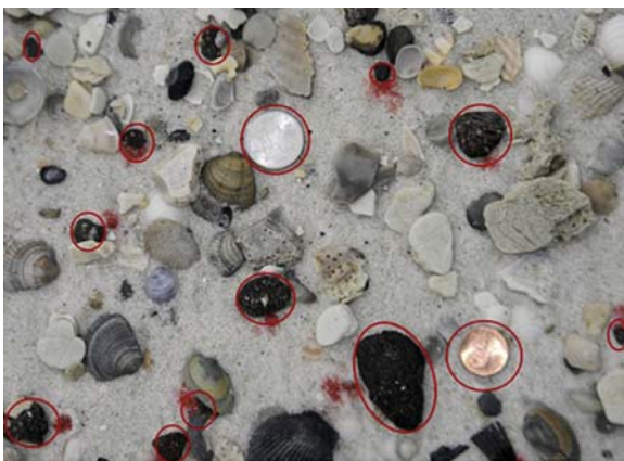
FIGURE 16.5 Typical SRBs mixed along with shells and other debris found in the swash zone. SRB locations are marked using red dye and SRBs are also circled; a quarter and a penny are used for scale. Photo taken near Lagoon Pass, Alabama, on February 19, 2012.
